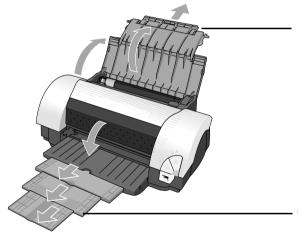
(1) Open the paper rest and pull out the paper rest extension to support the paper.
